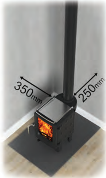
SINGLE WALL FLUE Rear Flue Configuration Back Wall: 250mm Side Wall: 350mm
