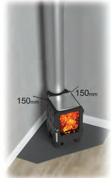
TWIN WALL FLUE Corner Configuration Left Side Wall: 150mm Right Side Wall: 150mm
